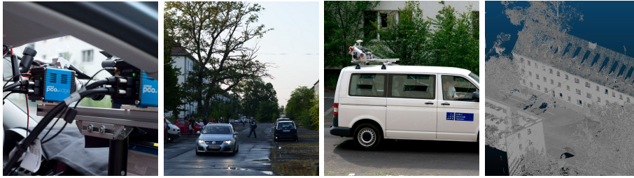
Fig. 3. From left to right: stereo rig, set photo, LIDAR mounted on car and resulting data.
